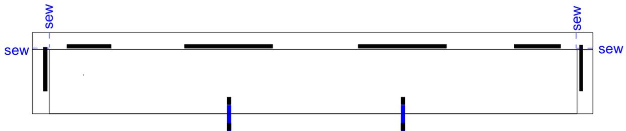
The following illustration shows how the curtain fits on the backdrop support with the H&L fastened together.
